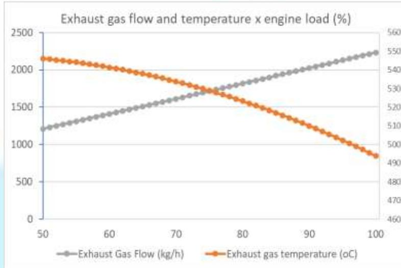
Figure 10 – engine part load exhaust gas flow (kg/h) and temperature (°C)
