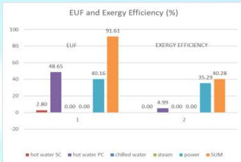
Figure 12 – EUF and exergy efficiency (heating mode)
