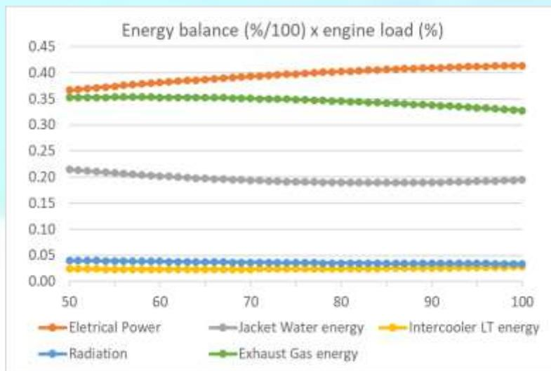
Figure 9 – engine part load energy balance
