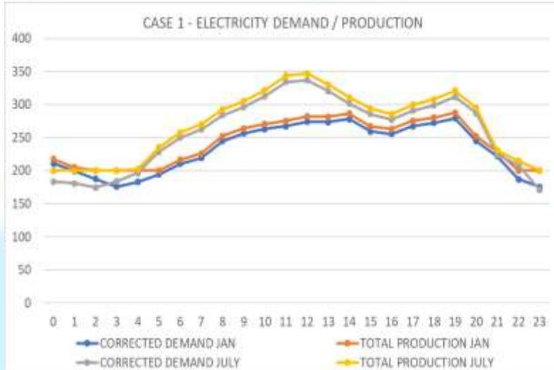
Figure 15 – case 1 electricity demand and production (kW) – January and July
