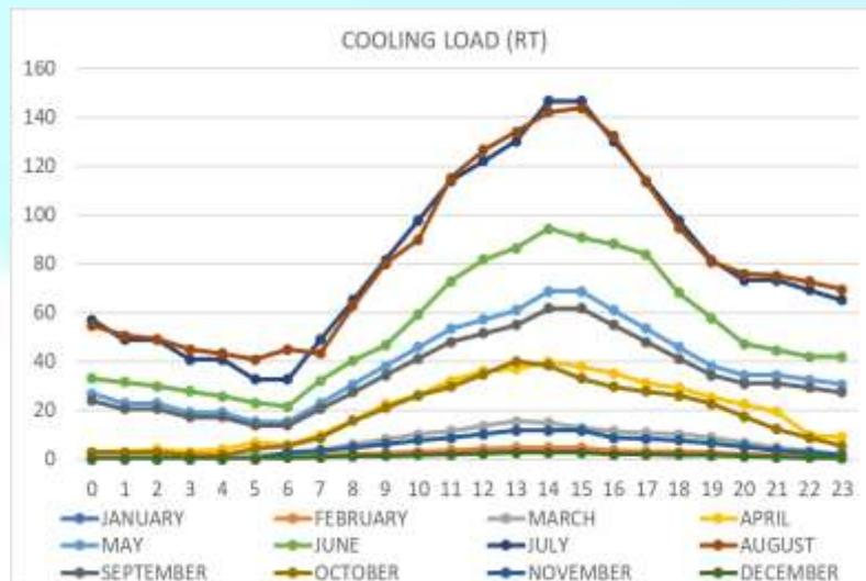
Figure 6 – hotel building cooling load (refrigeration tons)
