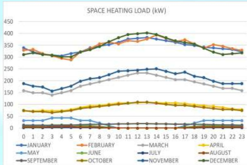
Figure 5 – hotel building heating load (kW)
