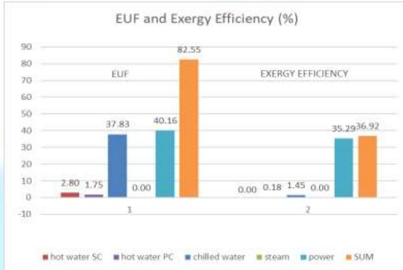
Figure 11 – EUF and exergy efficiency (cooling mode)
