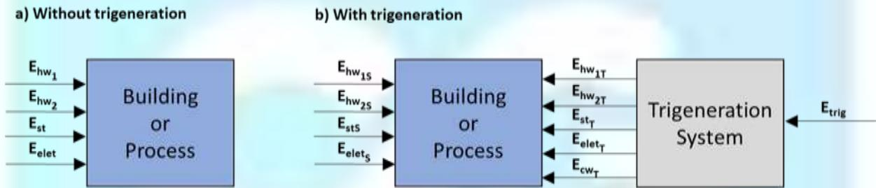
Figure 13 – building/process energy consumption
